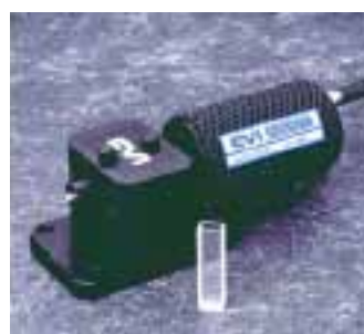
AT-SHC Fiber Optic Sample Holder (shown with a light source)
